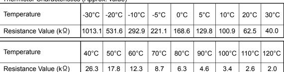
▶ If Thermistor is either open or shorted, replace it and reset the power.
